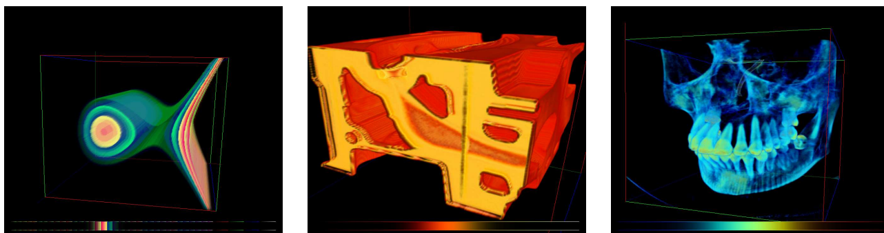
Figure 1: Tridimensional objects rendered as volume: (left) an implicit function close to its singularity, (middle) a tomography of two cylinders of an engine and (right) an x-ray scan of a human skull.
