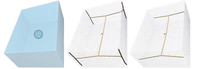
Figure 7: The result of our algorithm is a thin, 1D curve-skeleton even in degenerated cases such as a 3D box. When the initial model is not exactly centered (left), the skeleton quickly recovers the symmetry of the input (center). The filtering preserves the symmetry (right).
