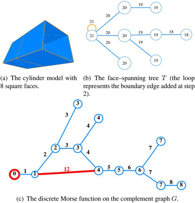
**Figure 5:** Algorithm's execution on a small cylinder model: 1 critical vertex and 1 critical edge with values 0 and 12.
