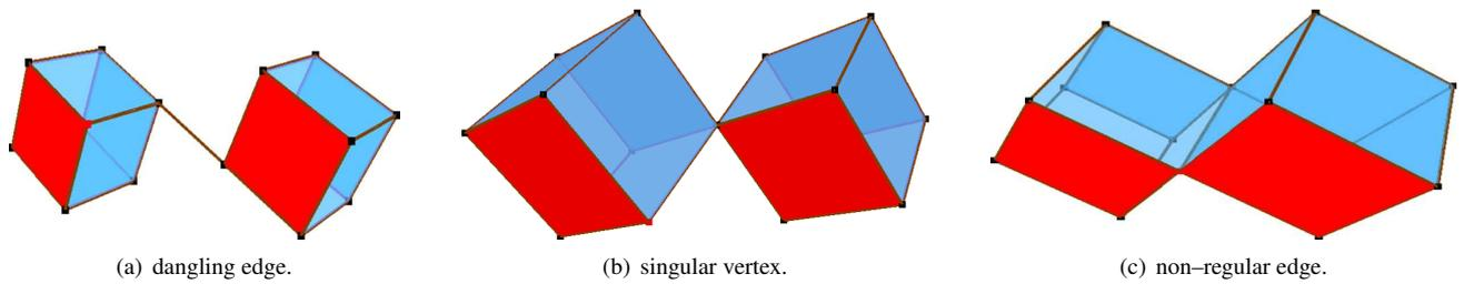
Figure 7: 3 non-manifold cases: 1 critical vertex and 2 critical faces (squares).
