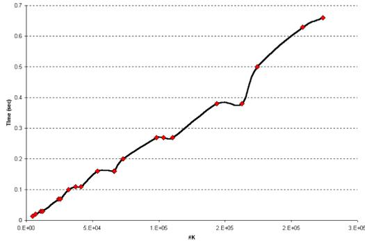
(a) Execution time versus the number of cells of the cell complex  $K$ : the complexity is linear.
